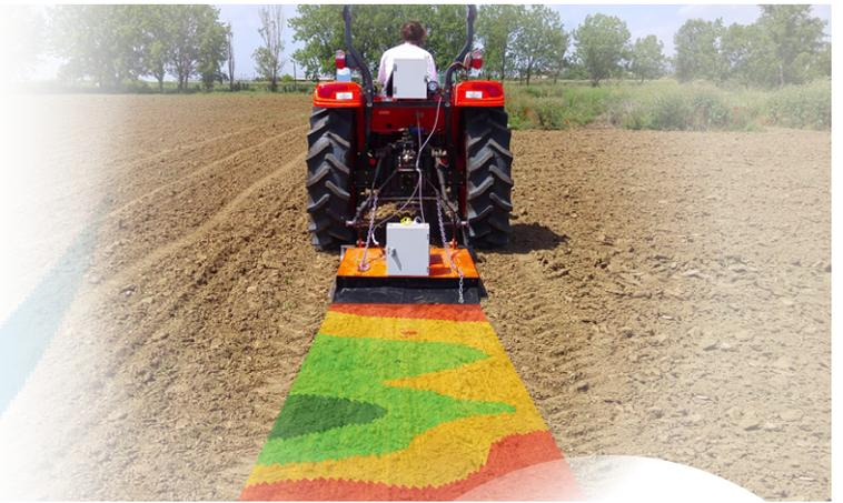
A system based on a mobile soil sensor measuring visible and near-infrared spectra developed to estimate spatio-temporal distribution of specific soil quality indicators
